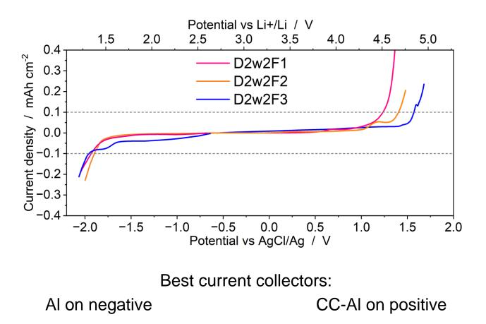
Linear Sweep Voltammetry measurement
