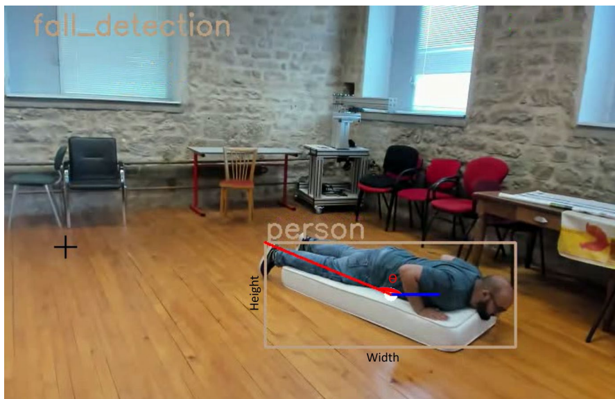
Fig. 6 Feature annotation on a sequence from our proprietary dataset: bounding box aspect ratio variation ( \delta = \text{height} - \text{width} ) and orientation angle ( \theta )
