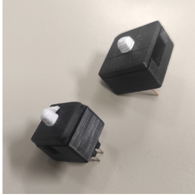
Figure 8.4: BaF 2 samples and their SiPM kept in place within black 3D-printed plastic holders. The detector on top, whose holder houses a Teflon-wrapped 3 × 3 × 10 mm 3 sample coupled to a 6 × 6 mm 2 SiPM, was measured in the 2022 testbeam, while the one on the bottom was tested in 2023 and is composed of a 2 × 2 × 10 mm 3 crystal coupled to a 3 × 3 mm 2 SiPM.
