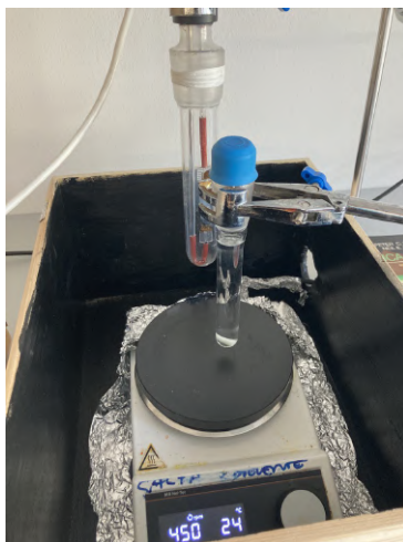
Figure 2.42 Photograph of the home made set up employed for photopolymerization under 254 nm irradiation.
