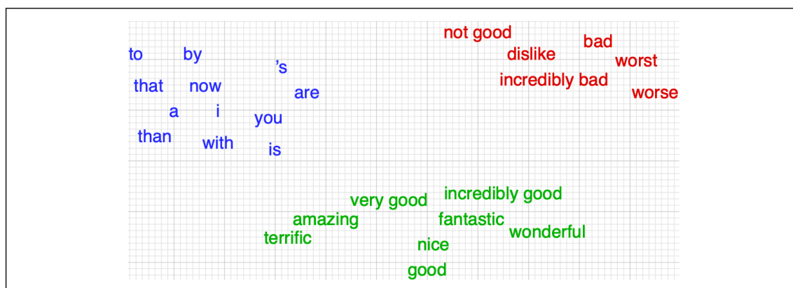
Figure 1.2: A two-dimensional (t-SNE) projection of embeddings for some words and phrases, showing that words with similar meanings are nearby in space. The original 60-dimensional embeddings were trained for sentiment analysis. Simplified from Li et al. [187] with color added for explanation.
