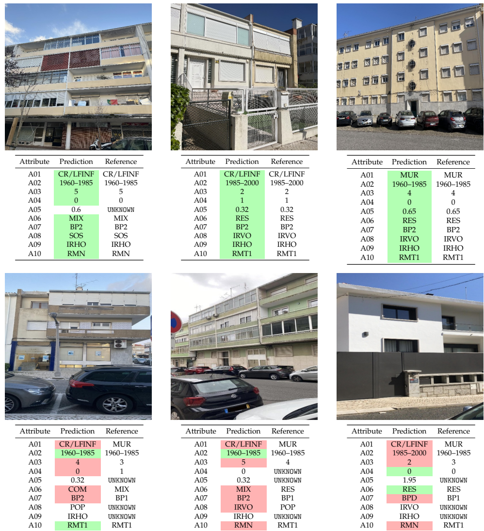
Figure 5. Examples of classification results from the top-performing model (DINO-v2 B). Attribute names correspond to those in Table 1. The top row shows a best-case scenario where all building attributes are correctly predicted. The bottom row shows a worst-case example with multiple misclassifications. Predicted labels are displayed alongside the corresponding reference values for comparison. Green and red colors highlight correct and wrong predictions, respectively.
