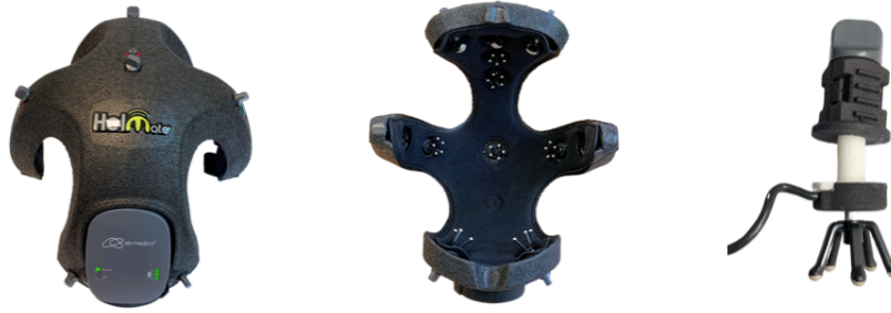
Figure 3.4: Electroencephalogram device Helmate8 from abmedica . From left to right: outside and inside of the device, a dry electrode.
