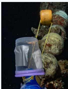
Figure 50 A - Non-destructive method through collection cups.
