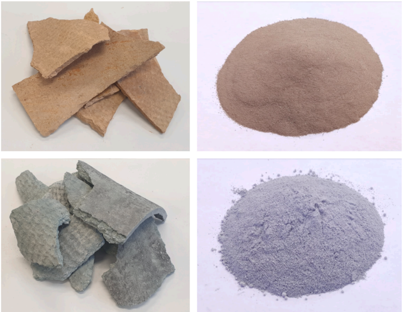
Fig. 1. Top: “Red” DAC; bottom: “Green” DAC; left: asbestos cements slates after thermal deactivation; right: powdered DAC.
