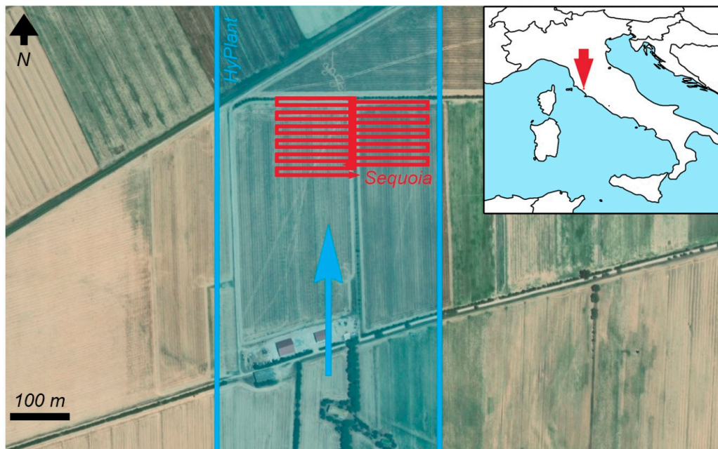
Figure 2. The studied maize field in the province of Grosseto, Italy is depicted along with its location (inset map). The flight lines and coverage of the drone (Sequoia, red) and airborne (HyPlant, blue) datasets are also shown. Image data licensed by ESRI, © DigitalGlobe.
