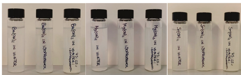
Figure 7. Redispersion of hydroxide in water, isopropanol, and 75:25 water/isopropanol mixture.
