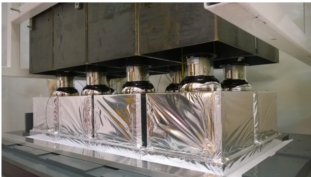
Figure 5. Picture of a calorimeter of 2x4 OMs during insertion of the pure iron magnetic shields.
