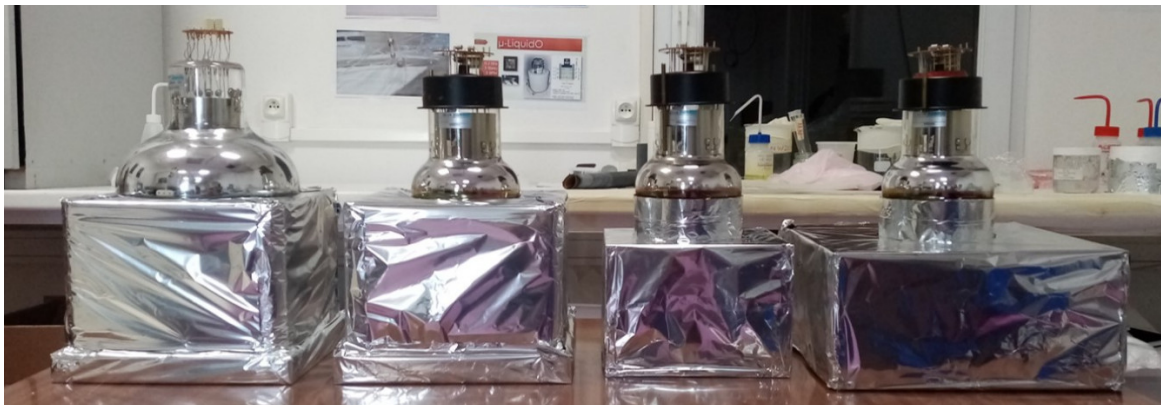
Figure 4. Picture of the four types of optical modules used for the SuperNEMO calorimeter during assembly. From left to right: two M-wall OMs with 8- and 5-inch PMTs, one X-wall OM and one G-veto OM with 5-inch PMTs and PMMA light-guide. Notice the wider step in the M-Wall scintillator block’s shape at the bottom of the corresponding OM. Scintillators and light-guides are wrapped with aluminized mylar.
