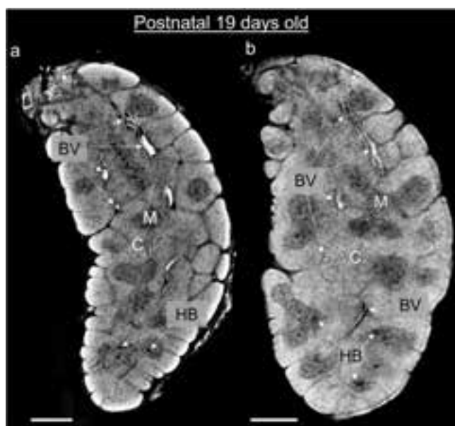
Fig. 7 | Laboratory-based CT solutions provide the same structural information as synchrotron equipment. Corresponding slices of a 19-day post-natal thymus acquired using SPC-CT (a) and H-CT (b). Both depict the same structural components of this sample, including cortex (C), medulla (M), Hassall's bodies (HB) and blood vessels (BV). Scale bars: 500 \mu\text{m} .
