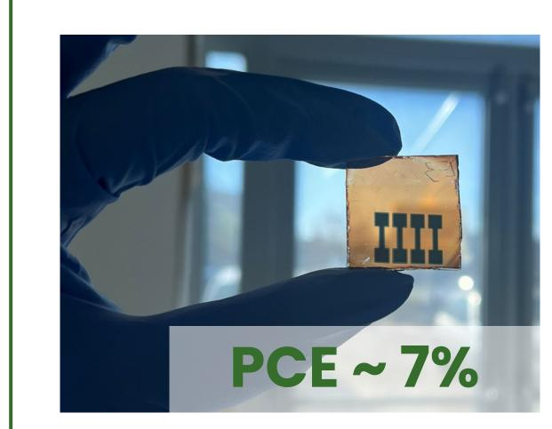
We have fabricated semi-transparent PSCs under ambient conditions, paving the way for their integration into building infrastructure, where they can simultaneously serve as windows and energy generators.
