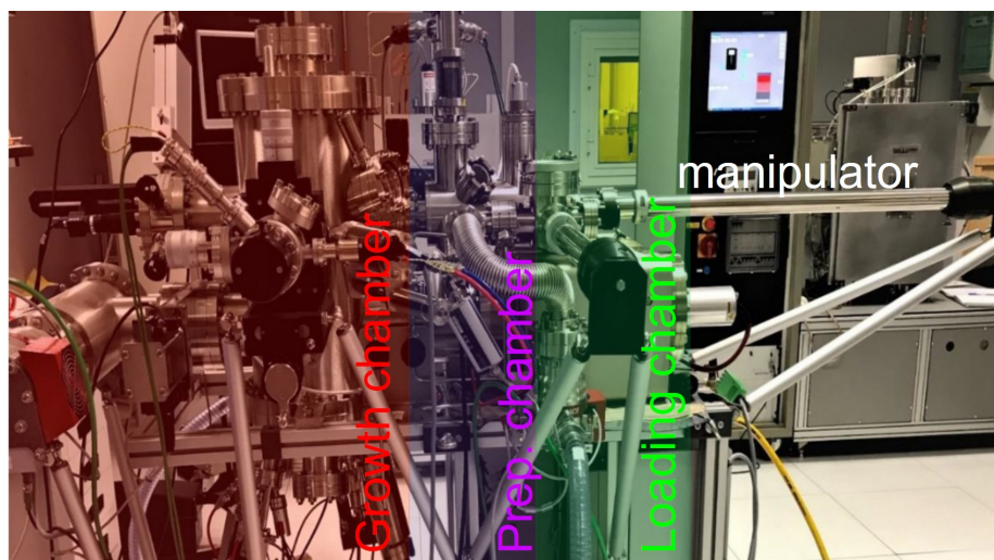
Fig. 3.2 Picture of the ScientaOmicron LAB10 MBE system used for the growth of Xenon on Ag(111) substrate.
