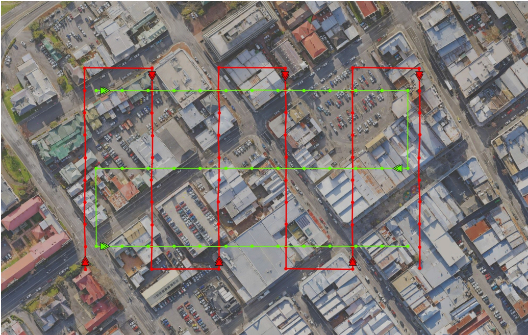
Figure 3.11: Camera paths on the ENRICH-Aerial dataset. In red the path followed by the first nadir and oblique cameras, in green the path followed by the second nadir camera.
