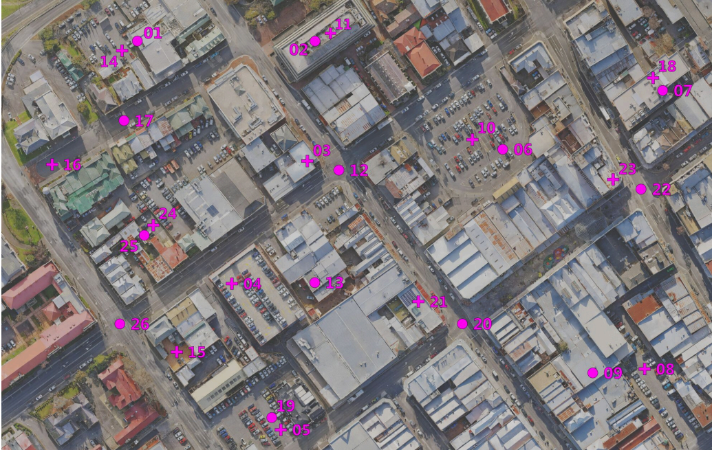
Figure 3.9: Orthographic view of the GCPs placement on the ENRICH-Aerial dataset. Cross and round shapes as in Figure 3.4.
