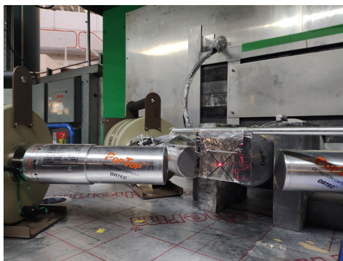
Figure 5.6: Experimental setup. The laser spot serves as a reference system to place the sample at the right height.
