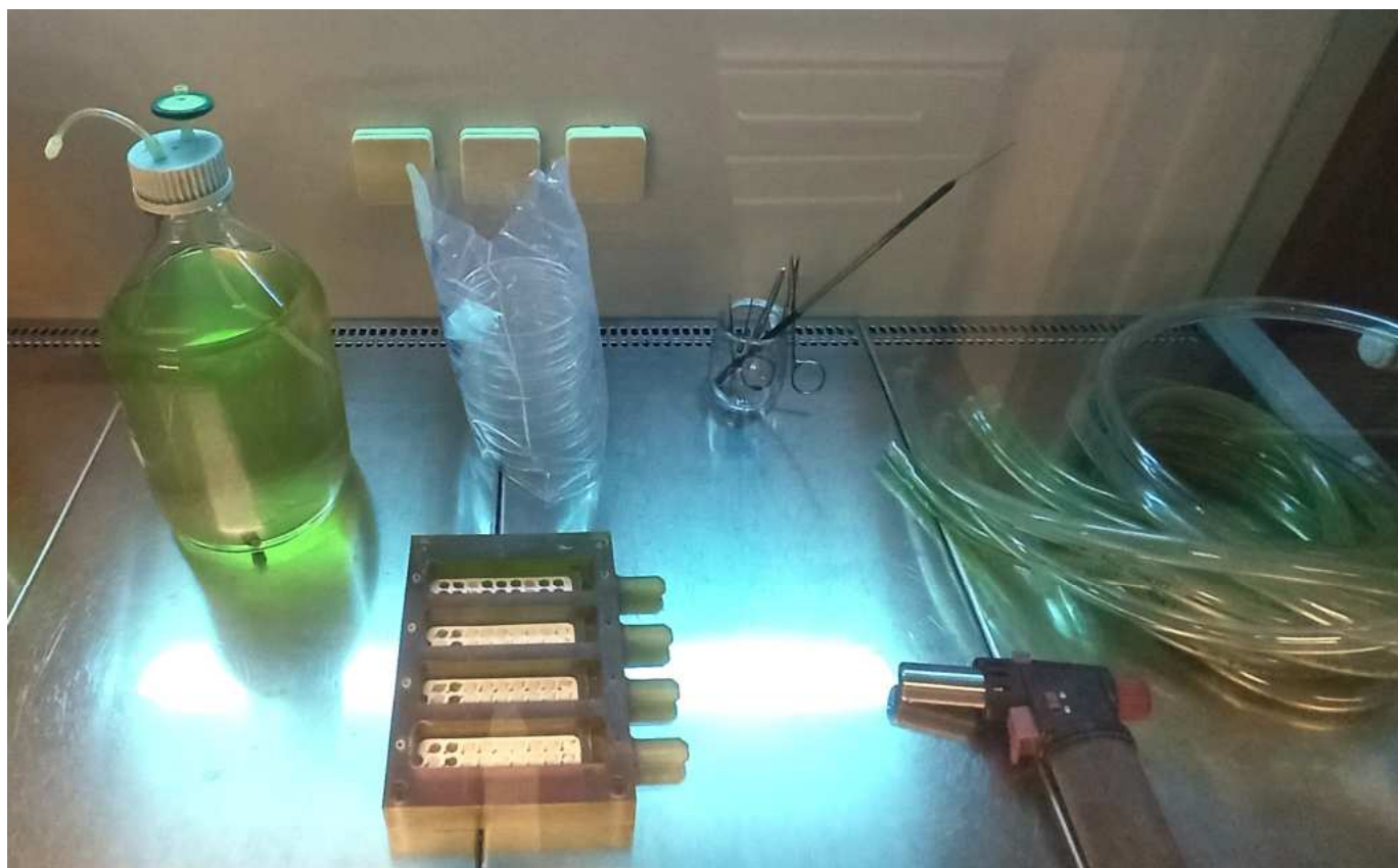
Figure 2. The M-DFR bioreactor prior to final assembly inside the sterile hood under UV irradiation. Its main body contains the enamel disks kept at the bottom of the parallel flow cells by the polytetrafluoroethylene customized specimen trays (white). The sterilized modified artificial saliva medium is seen on the left, while the tubing leading to the waste outside the incubator is shown on the right.
