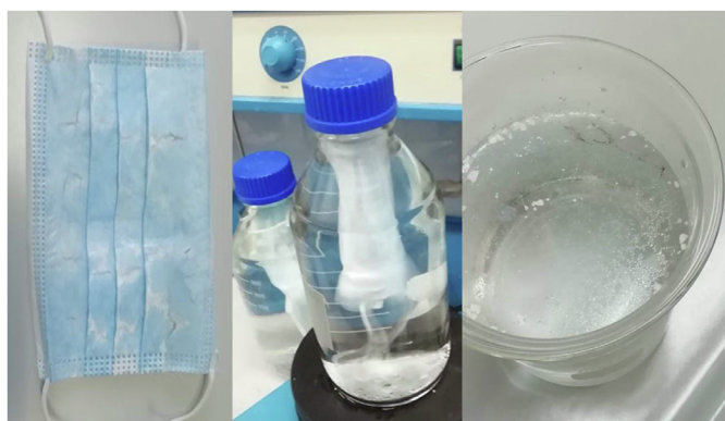
Fig. 1. Pictures from the experimental procedure. From the left to the right: (a) a surgical mask after prolonged UV light exposition (b) surgical mask stirred inside a bottle filled with artificial seawater solution (c) appearance of the microfibrers “soup” on the top of the artificial seawater solution at the end of the artificial weathering treatment.
