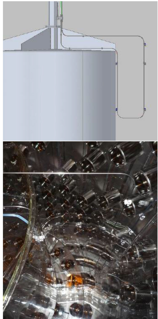
Fig. 25 The guide tube system used to calibrate the detector in the top half of the GC
