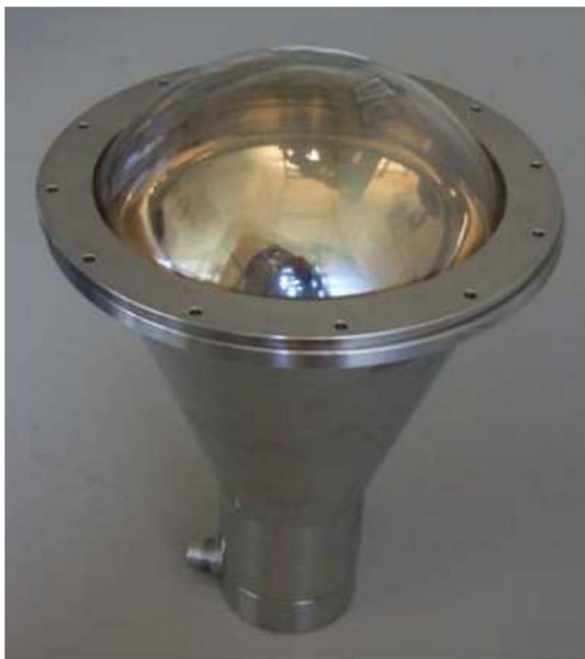
Fig. 17 Stainless steel enclosure with a transparent PET window, an oil-tight cable feedthrough, mu-metal shielding, the Hamamatsu R1408 PMT, and the PMT base. The inner volume was filled with mineral oil
