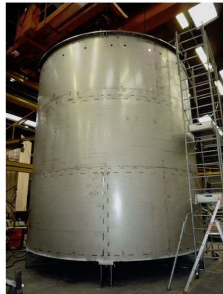
Fig. 3 Technical drawing (top) and photograph (bottom) of the Double Chooz Buffer vessel, composed of a frame made of stiffening profiles (1565 kg) on which a “skin” made of 3 mm thick steel sheets (4500 kg) was fixed. It rested on 6 feet (3525 kg) and supported the 390 photomultiplier tubes, drain and expansion tubes
