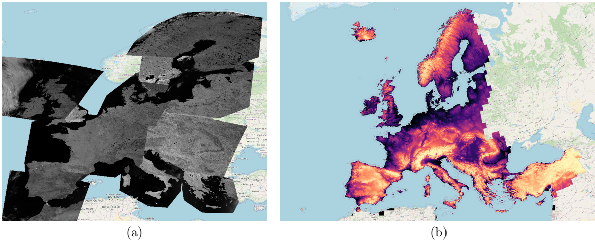
Figure 6.1: Representation of the data used in these experiments. (a) shows multispectral images collected by Sentinel-3 and properly merged to cover the entire European continent. For the sake of visualization, (a) represents the average over all the bands, normalized between 0 and 1. (b) represents the digital elevation model acquired from the Copernicus Land Monitoring Service. Greenish colours represent low-elevation values (approx. -214 m), while reddish colours represent high-elevation values (approx. 5105 m).
