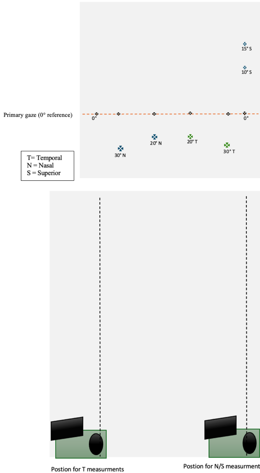
Figure 4. 6 Schematic representation of the peripheral refraction measurement setup and fixation geometry. Positions are schematic and not drawn to spatial scale
