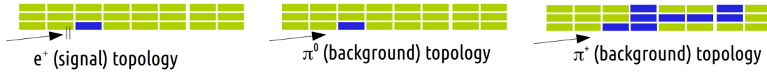
Figure 2.8: Energy deposition topologies for electromagnetic and hadronic showers in the longitudinally segmented calorimeter.
