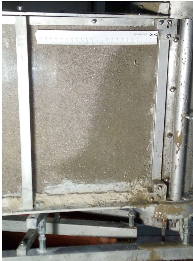
Figure 15: detail of injection test carried out with ITS 1.0, the progress of the mix in the soil and the losses at the triple points can be seen.
