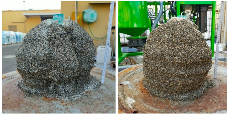
Figure 40: cemented soil bulb
