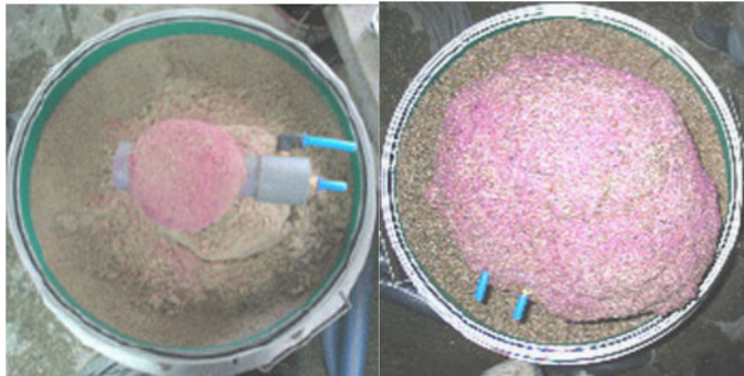
Figure 10: grouted sand bulb of the two different soils.
