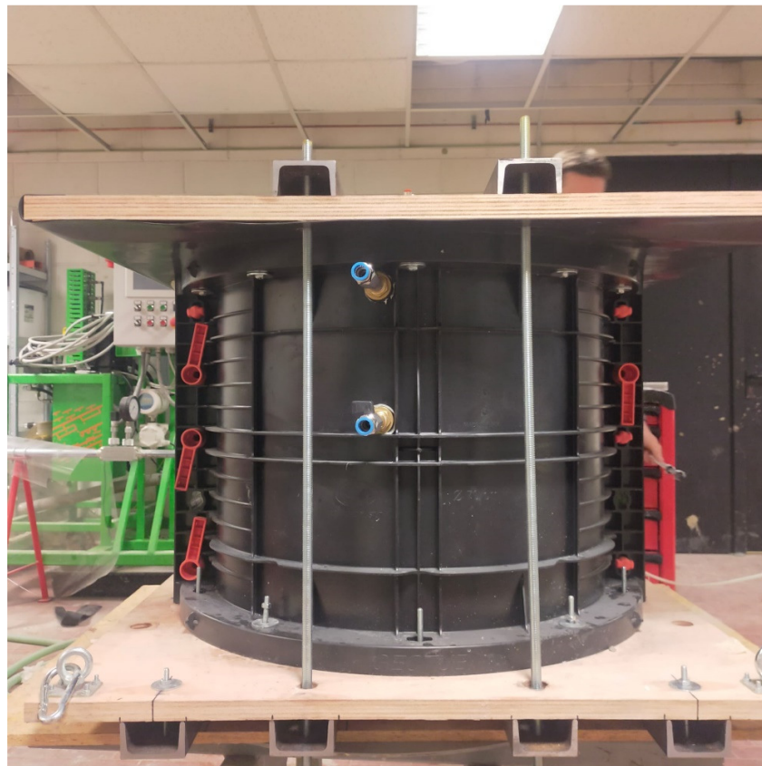
Figure 4: modified cylindrical apparatus with new top and bottom, iron beam and drainage system.
