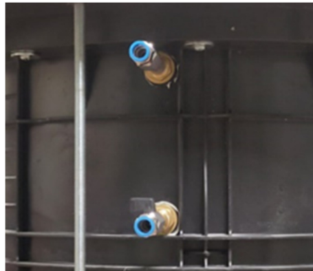
Figure 8: detail of the drains on the cylindrical formwork that allow the water saturating the soil sample to be pressurised and drained during the injection phase.
