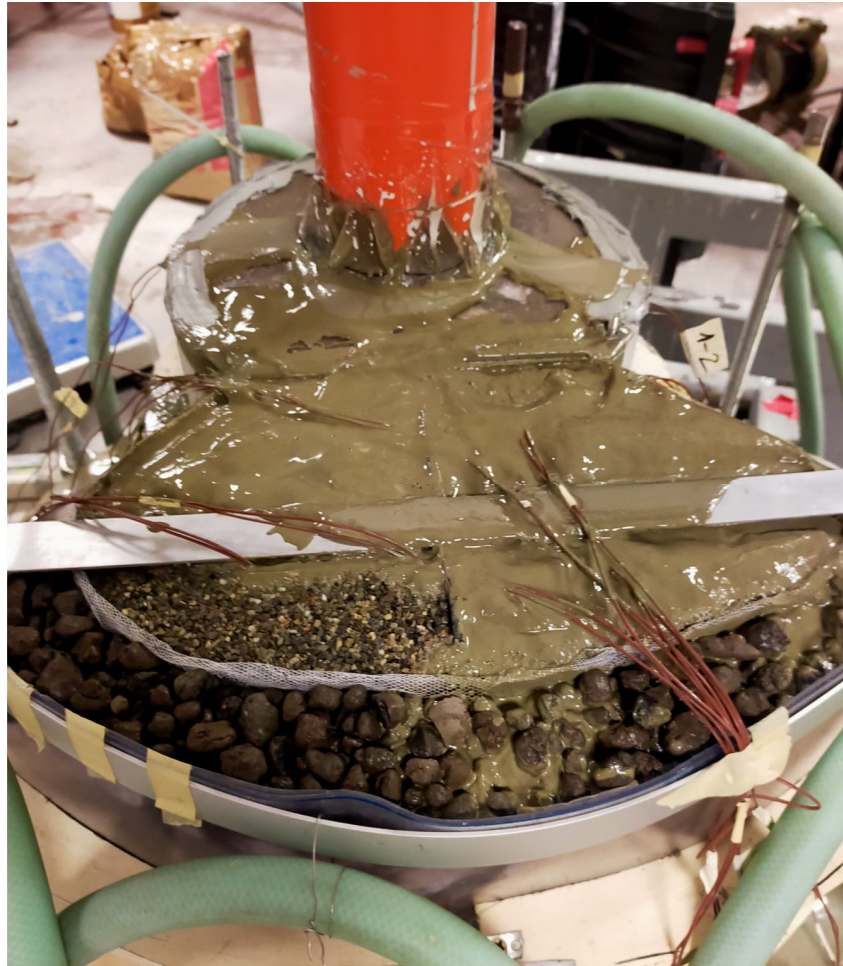
Figure 18: mixture leakage from the top of prototype
