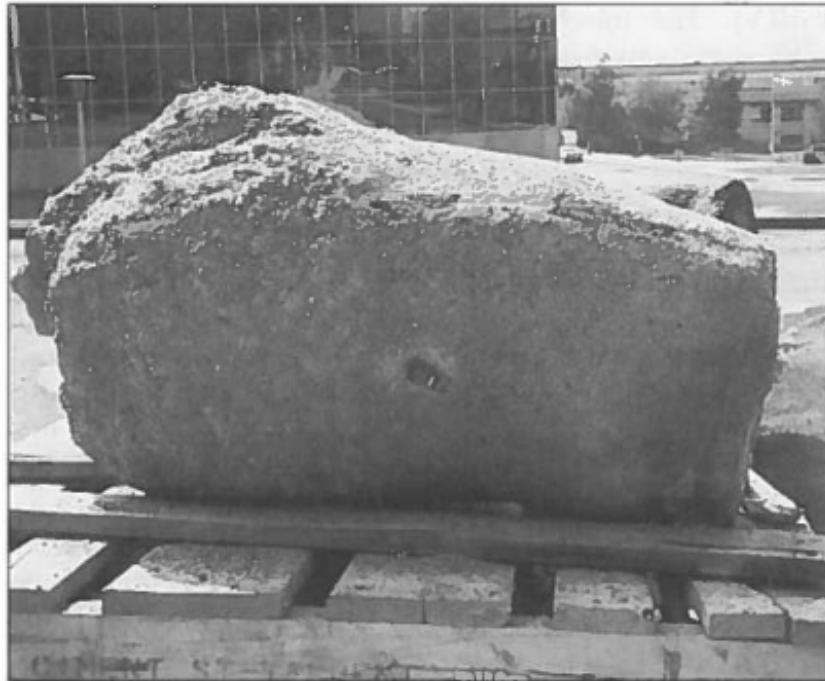
Figure 6: saturated alluvial sand after injection (Perret,2000)
