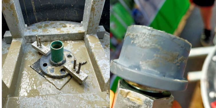
Figure 23: TAM without cap (on the left), the cap detached from the mixture pressure (on the right)
