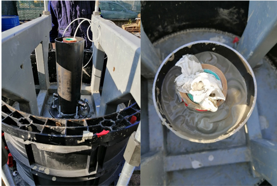
Figure 33: metal flange for augmented bentonite sheath load
