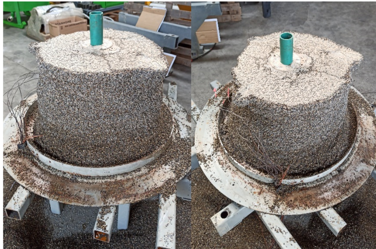
Figure 29: cemented soil volume
