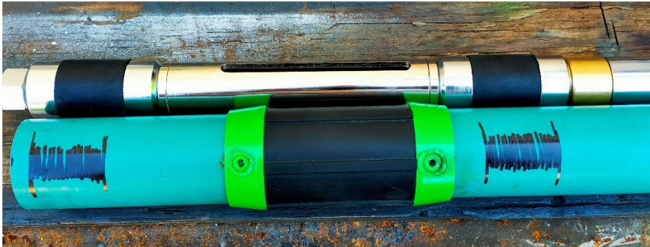
Figure 24: double packer and a tube a manchettes
