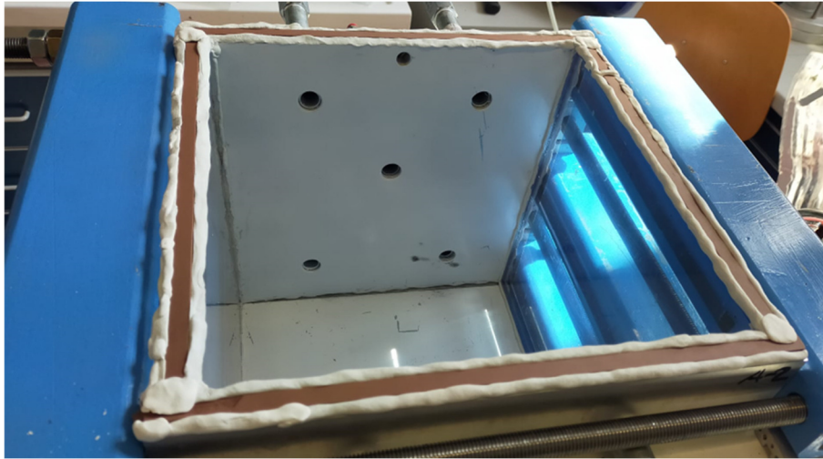
Figure 12: materials used as a gasket between the constituent parts of the SquaCol.
