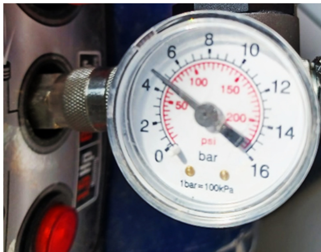
Figure 11: maximum pressure reached inside SquaCol; the hydraulic seal has been checked.
