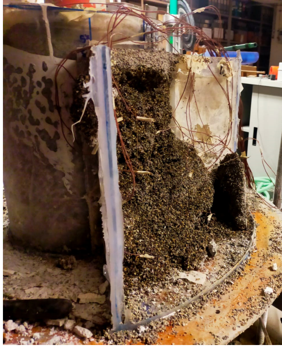
Figure 19: bulb of soil after cement mixture injection
