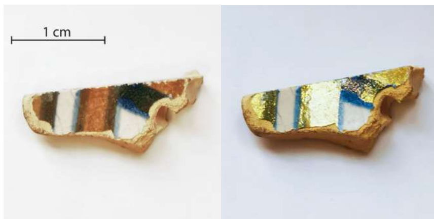
Figure 6.9: Sample analyzed at the XRF line of the Elettra synchrotron, the lustered part investigated is the central golden stripe.
