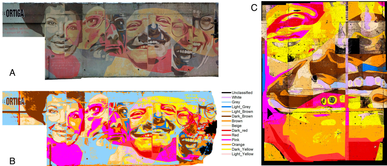
Fig. 7. Comparison of the SAM results. (A) Orthophoto mosaic and (B) corresponding SAM results for the MSI dataset compared with (C) the SAM results of the HSI dataset. Color legend and sampling positions of the endmembers are the same for the two datasets.
