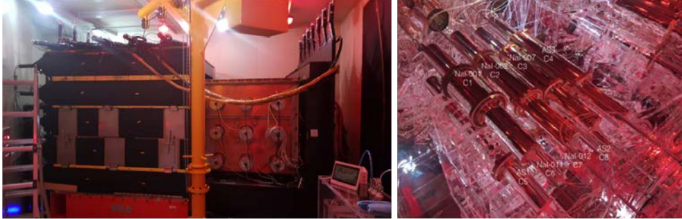
Figure 1: Left : Side view of the COSINE detector. Outermost we installed 37 plastic scintillator panels to tag muon with 4\pi coverage. Each panel, we attached one (or two for only top panel) 2-inch PMTs. Inside muon detector panels, we have 20-cm-thick lead shielding, and 3-cm-thick copper box. Inside the copper box, we installed LS veto that will contain \sim 2000 L of LS inside acrylic box which will be shown with 18, 5-inch PMTs. Right : We installed NaI(Tl) crystals, a 4 \times 2 array, inside acrylic box. Two, 3-inch PMTs were attached at each side of individual crystal. NaI(Tl) crystal is hygroscopic, so each crystal was encapsulated with copper to prevent any contact with air. PMTs also sealed with copper end cap to prevent any leakage when immersed into LS. We attached vikuiti sheet on copper surface and inner surface of acrylic box to increase light collection efficiency of LS veto layer.
