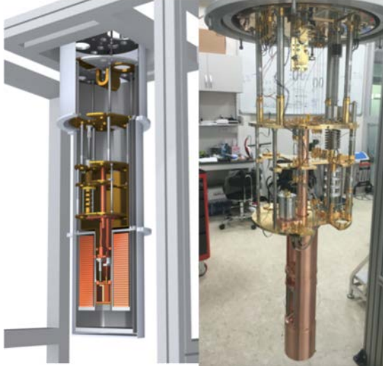
Figure 3: BlueFors LD400 dilution refrigerator with cavity and frequency tuning system installed
