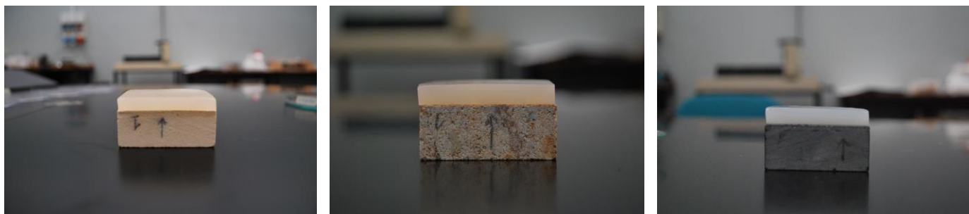
Figure 9. From left to right: Noto calcarenite, Manciano sandstone, Bergamo black limestone with rigid Bresciani agar gel 3%.
