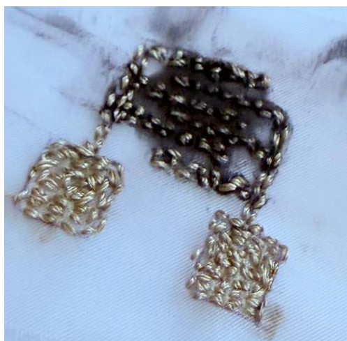
Figure 6. 14 Photograph of the Embroidered IDE-rGO/CuO Gas Sensor
