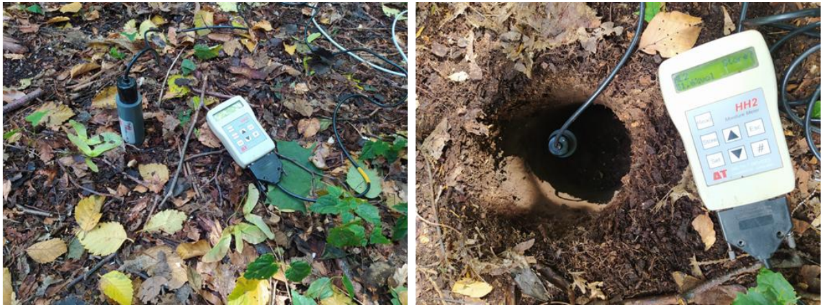
Figure 36: use of the ThetaProbe for in situ measurement of soil moisture content.
