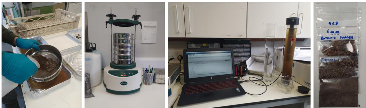
Figure 37: PSD experimental setup: Sieving and densimeter..
