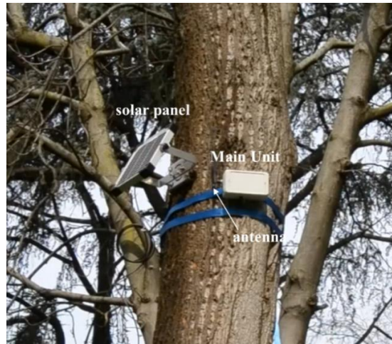
Figure 110: Main Unit with solar panel integrated.
