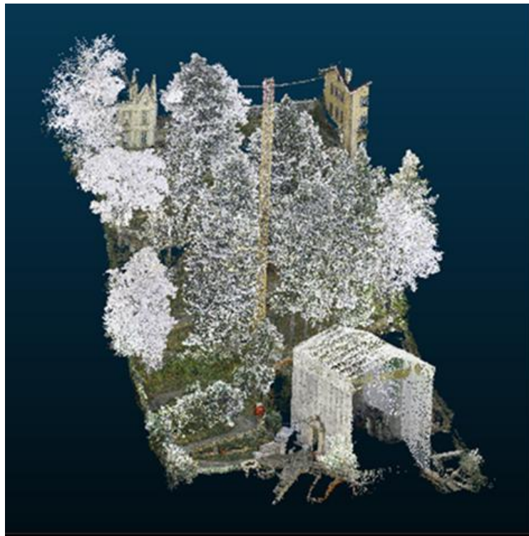
Figure 120: point cloud of property of Villa Springwater acquired by GeoSLAM ZEB.
