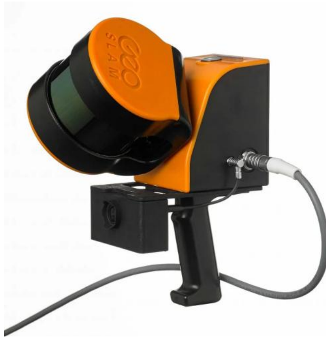
Figure 118: Handheld GeoSLAM ZEB Horizon LiDAR scanner used for mobile 3D point-cloud acquisition and SLAM-based reconstruction of the tree and its surroundings.
