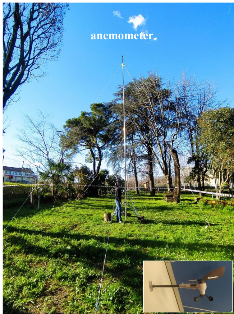
Figure 108: anemometer installed at the Vivavio Bicocca.
