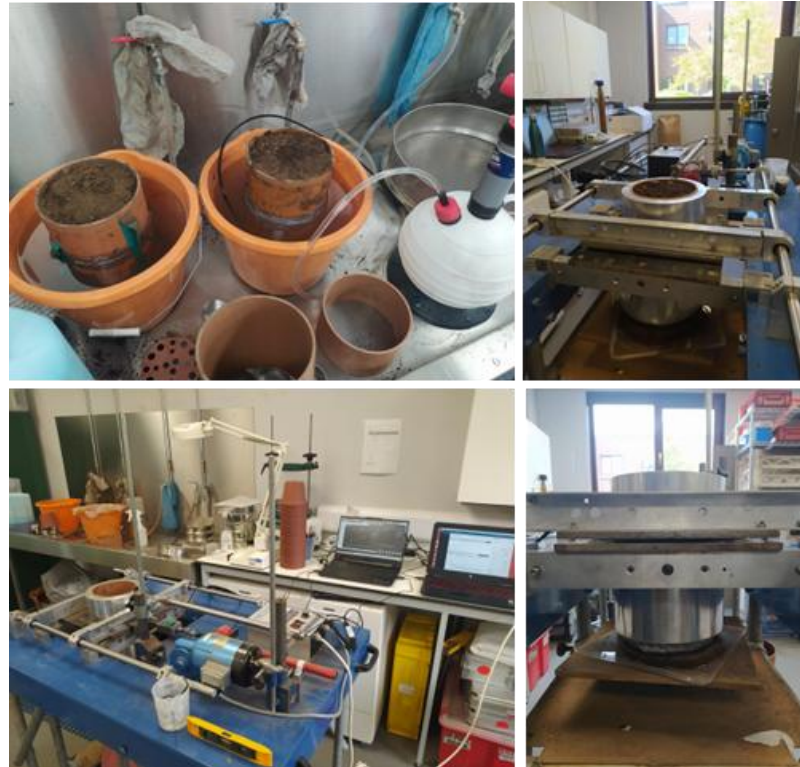
Figure 41: direct shear testing setup.
