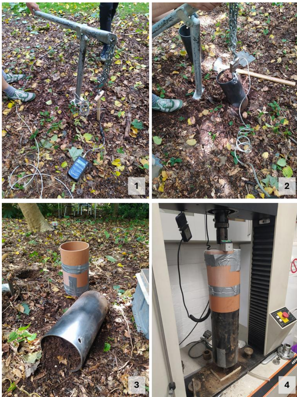
Figure 40: tube sampling procedure for direct shear tests.
