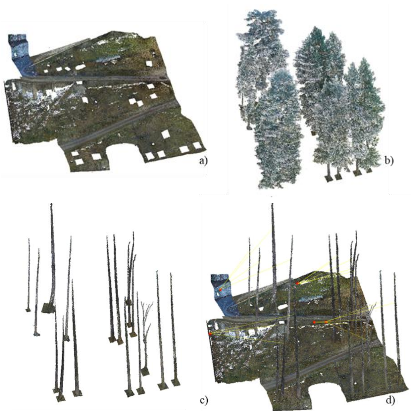
Figure 123: a) cleaned slope, b) trees (collars, trunks and crowns, c) collars and trunks, d) slope and trees without crown with anchoring points on the ground (red dots) and guiding rope (yellow lines).
