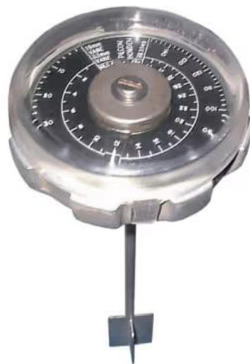
Figure 35: vane test apparatus used in the field test campaign.
