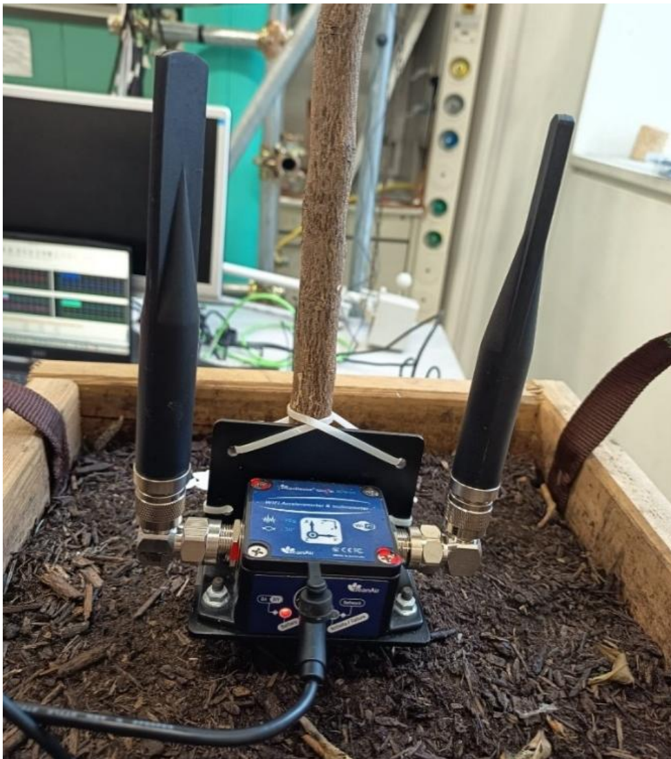
Figure 82: inclinometer/accelerometer with high gain antennas mounted on the collar of the tree.
