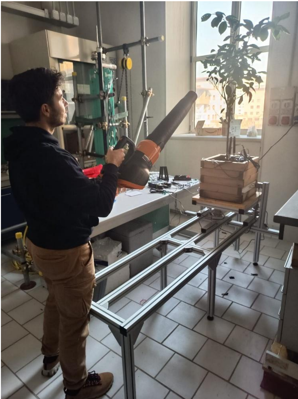
Figure 83: methods of blowing the tree canopy. A portable blower can be directed according to the type of test to be performed.
