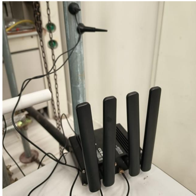
Figure 88: Teltonika Networks RUTM54 industrial router used for the 2.4 GHz WLAN connection in laboratory tests.
