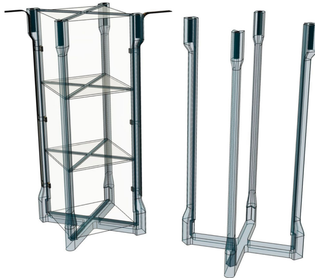
Fig. 7 Design of monolithic structure, manufactured as a single unit. Crystals are stacked inside the structure separated by thin spacers. As the structure shortens during cool-down the dimensional tolerances are a critical aspect of the engineering process. The collection of the scintillation light is facilitated by the uninterrupted design of the vertical columns and light sensors can be placed either at the top of the tower, or even remotely and the photons collected and transported by means of optical fibres
