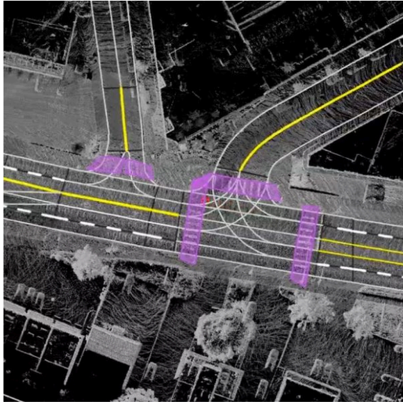
Figure 2.6: Example of a an HD map providing both geometric data and high level information of the navigation environment. Image taken from [187].
