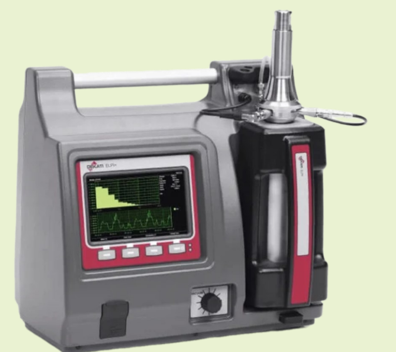
Figure 4. Dekati ELPI+ (Electrical Low-Pressure Impactor) particle size spectrometer.
