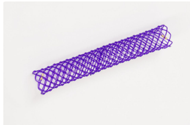
Fig. 2 Macroscopic appearance of the self-expandable stent made of polydioxanone monofilament braided to form an uncovered mesh, with gold radiopaque markers at the extremities
