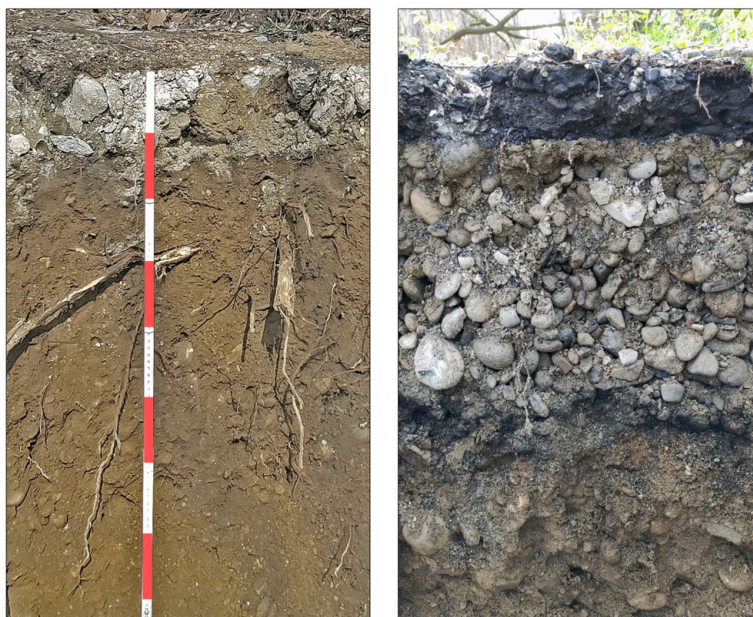
Figure 13. Soil sealed by asphalt and concrete. On the left, the roots in the sealed soil come from trees growing by the roadside. On the right, the removal of the fertile layer (topsoil) and the addition of a subgrade are clearly visible, leaving only the mineral soil substrate in evidence.
