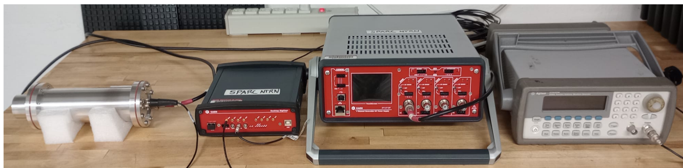
FIG. 3. Prototype of the SPARC HXR monitor: LaBr 3 crystal + PMT enclosed in an aluminum case, CAEN DT5730s digitizer, CAEN DT1471ET high-voltage module, and Agilent 33220A pulse generator.
