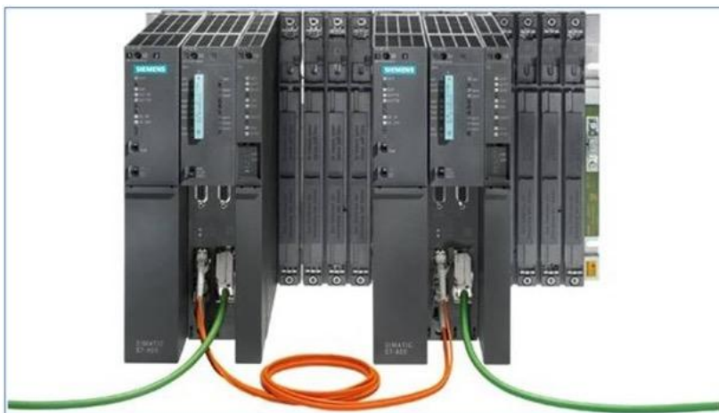
Figure 51. Redundant Siemens S7-400 PLCs.
