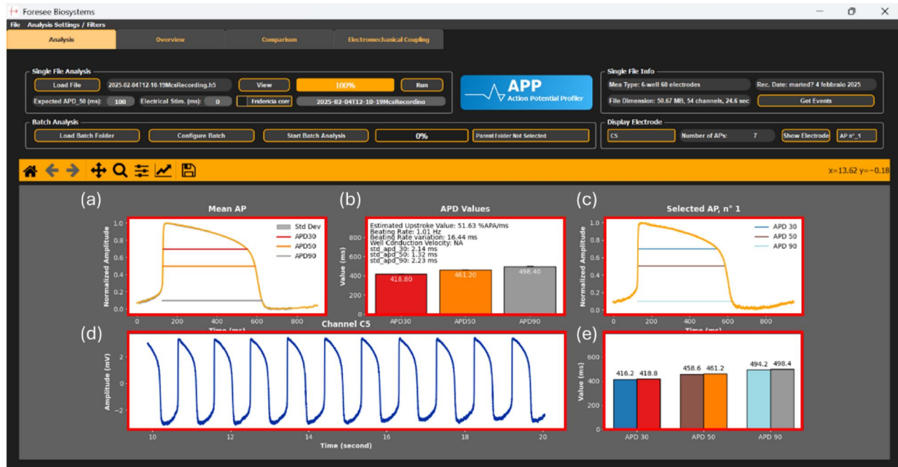
FIG. 6. Main window of the analysis software Action Potential Profiler (APP). The red squares highlight the main results of the analysis of APs acquired with IntraCell and MEA systems. (a) Mean AP of the selected electrode, normalized; (b) main parameters of the mean AP, including APD 30 , APD 50 , and APD 90 , estimated upstroke velocity, beating rate, and standard deviations; (c) specific AP selected in the analyzed electrode trace, normalized; (d) time course of APs from the selected electrode; and (e) comparison between the mean AP and the selected AP.
