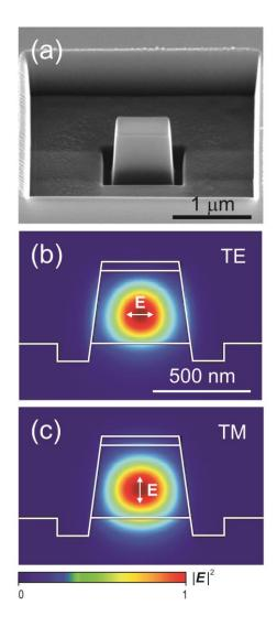
**Figure 1.** (a) SEM image of a Ge nanoresonator. The thin oxide protective layer and the slightly tilted lateral walls, due to the FIB beam profile, are also visible. (b) Field intensity map of the lowest-order (b) quasi-TE and (c) quasi-TM mode in the Ge waveguide, calculated by FDFD on a model structure closely resembling the nanoresonators under study.
