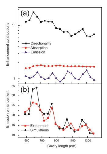
**Figure 3.** (a) Individual contributions to the total enhancement obtained from simulation results: increase in the absorbed power per unit volume (red line, circles), emission enhancement (blue line, triangles), and directional emission (black line, squares). (b) Results of FDTD simulations for the total enhancement per unit volume (black line, circles) and their quantitative comparison with the experimental results (red line, squares).
