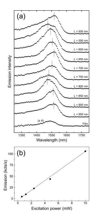
**Figure 5.** (a) Experimental room-temperature photoluminescence spectra from individual Ge nanoresonators and from the reference continuous Ge film, acquired with the same excitation power. (b) Representative emission rate from a resonant cavity as a function of the excitation power.
