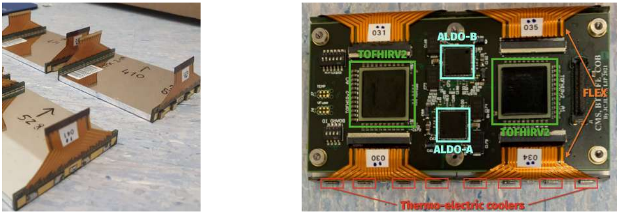
Figure 6.10: Left: A BTL array of 16 LYSO:Ce bars wrapped with a ESR foil and glued on both ends with SiPMs. SiPMs are connected to flex circuits for the connection to TOFHIR (orange). Right: the BTL front-end board with two TOFHIR2 chips (green), each connected through the 32 flexes (orange) to the SiPMs, two ALDO2 chips each serving one TOFHIR (cyan). Four TECs (red) are installed back-to-back with the SiPM array. One TEC serves 4 SiPMs.
