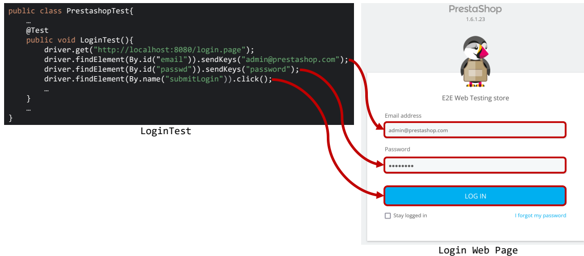
Figure 1: A Selenium login test script (left) and the corresponding login Web page under test (right).
