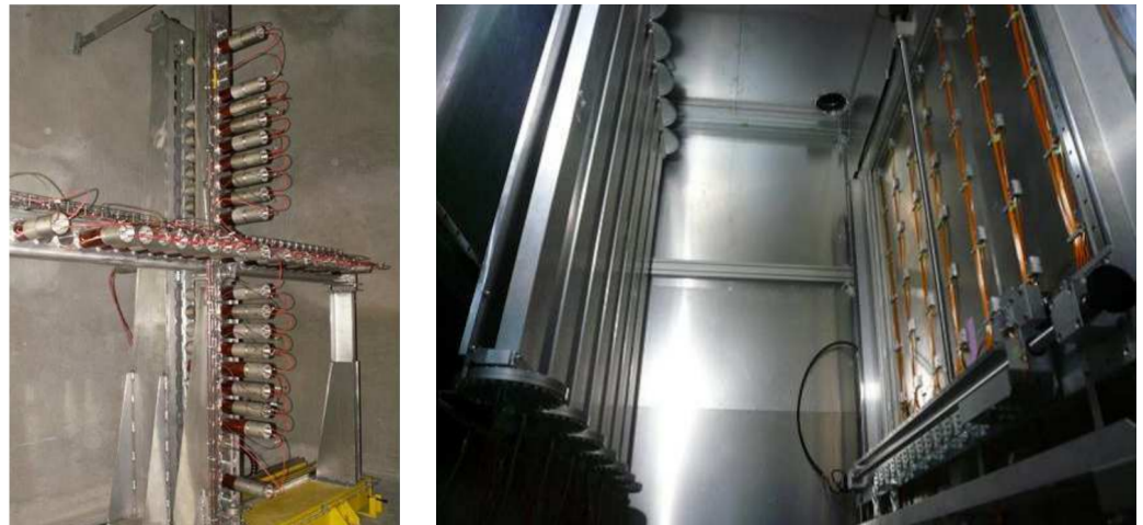
Figure 13. Muon monitoring detectors employed for the CNGS neutrino beam (left) and the J-PARC beam (right). The CNGS chambers consisted of 42 muon detectors separated by 11.25 cm and spanning a length of 2.7 m. The J-PARC system (MUMON) is composed of 7 \times 7 ionization chambers (left side of the picture) and 7 \times 7 , 1 \text{ cm}^2 , PIN photodiodes (right side). The beam enters from the right side. Reproduced under CCA4.0-I license with permission from Sissa-Medialab [28].
