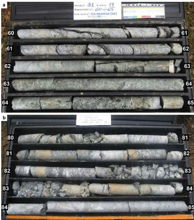
Fig. 6 - Core samples resulting from drilling in the Branega Fault Zone. a) Core samples of drill hole B1 taken at depth between 60 and 65 metres in the Branega Valley: at about 62.30 m depth, foliated cataclastic calc-schists make a transition to the underlying brecciated serpentinites (Acquasanta breccia); b) Core samples of drill hole SGG6 taken at depth between 80 and 85 metres: a calc-schist tectonic breccia and a gouge underlie brecciated serpentinites.
