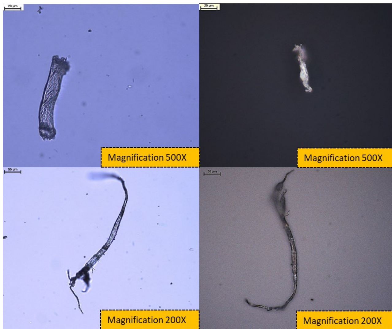
Figure 4cii – Enlarged microscope images of detected fibres. Scale bar: 20 µm corresponds to 500× magnification; 50 µm corresponds to 200× magnification.
