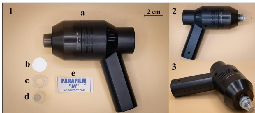
Fig. S1. Assemblage of the E-PoS a . 1. Overview of all the materials needed for the assembly of the E-PoS a device (a. Portable vacuum; b. Paper filter with 25 µm pore size; c. 5 mL Eppendorf tube's cap drilled; d. 5 mL Eppendorf tube with Stainless steel mesh with 75 µm mesh size at the tip; e. strip of laboratory film); 2. Top view of the fully assembled E-PoS a 3. Frontal view of the fully assembled E-PoS a .
