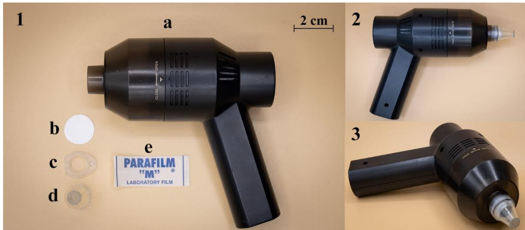
Figure 1. Assemblage of the E-PoSa. Overview of all the materials needed for the assembly of the E-PoSa device (a. Portable vacuum; b. Paper filter with 25 \mu m pore size; c. 5 mL Eppendorf tube's cap drilled; d. 5 mL Eppendorf tube with Stainless steel mesh with 75 \mu m mesh size at the tip; e. strip of laboratory film); 2. Top view of the fully assembled E-PoSa 3. Frontal view of the fully assembled E-PoSa.
