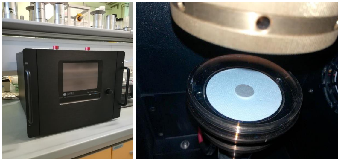
Figure 18. TCA08 analyzer used for TSP samples (a); punched filter over the installed 47mm filter (b).
