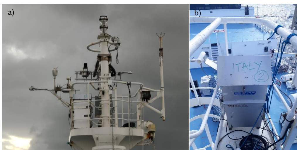
Figure 7. Small balcony at the end of the atmospheric mast (a). High volume sampler (b).
