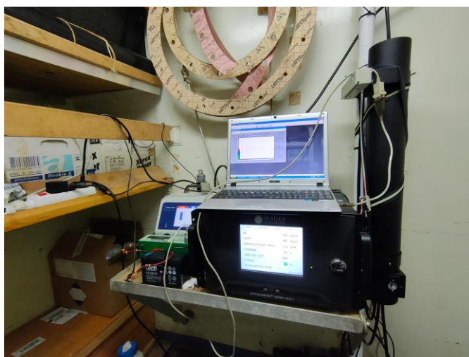
Figure 6. Instruments (AE33, OPC and NanoScan) installed inside the dedicated room
