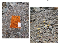
painted pebble surface for bedload monitoring
