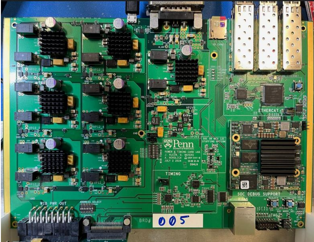
Figure 17. Revised PTC containing new functions relative to the ProtoDUNE-HD PTCs. The connections to the PTB are through the connectors shown in the bottom left, and front panel connections to external systems are at the top.
