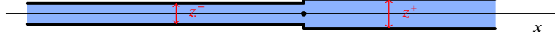
Fig. 2 Pipe with a discontinuity in the cross section, z^- being the cross section of the pipe to the left of the discontinuity and z^+ the cross section to the right.
