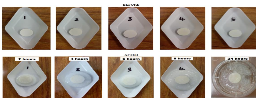
Figure 3. Swelling behavior comparison for bilayer tablets in 2% SDS aqueous solution (pH 4.2), at different time intervals.
